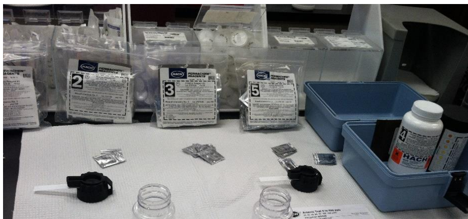
Figure 2: Arsenic Testing Kit and Setup
